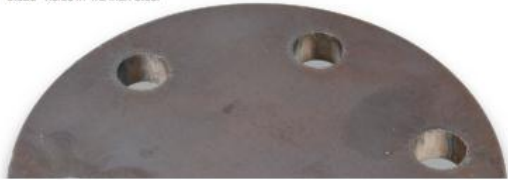
5/8 inch bolts in the above holes (top of part)
